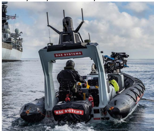
Uncrewed pacific 24 Rigid Inflatable Boat by NavyX and BAE Systems.
